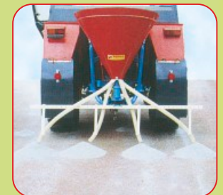
ADDITIONAL EQUIPMENT TO SPREAD FERTILIZER IN 4 ROWS
